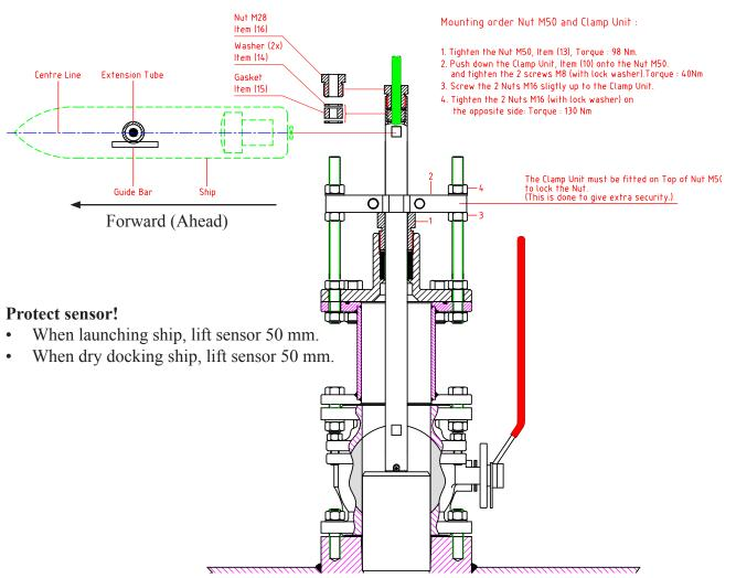
Check that the transducer sensor housing, when fully inserted, is flush with the lower surface of the bottom flange.
